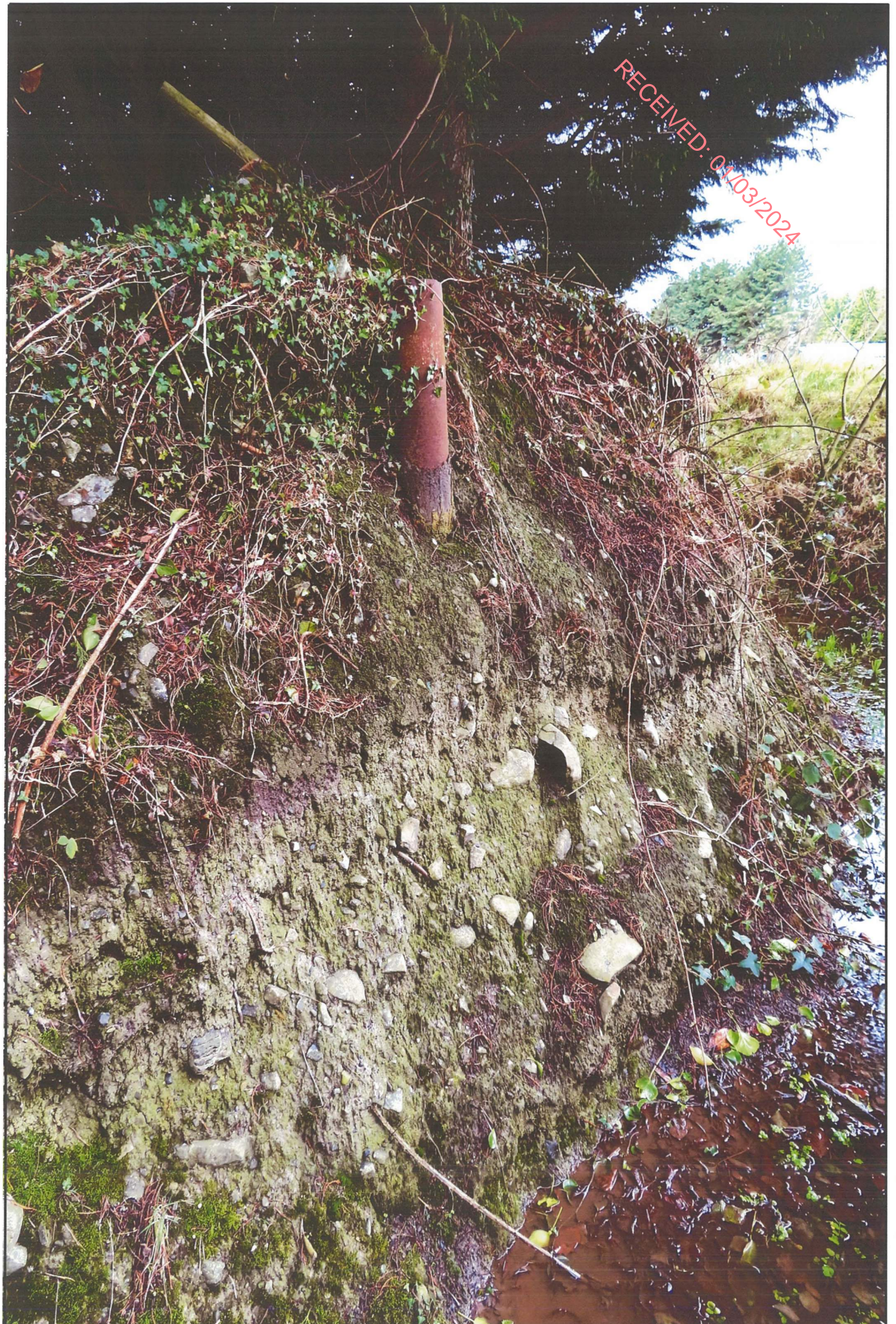
Figure 5.7 Borehole SG6, Exposure of Till and deep perimeter drain 5th February 2021
